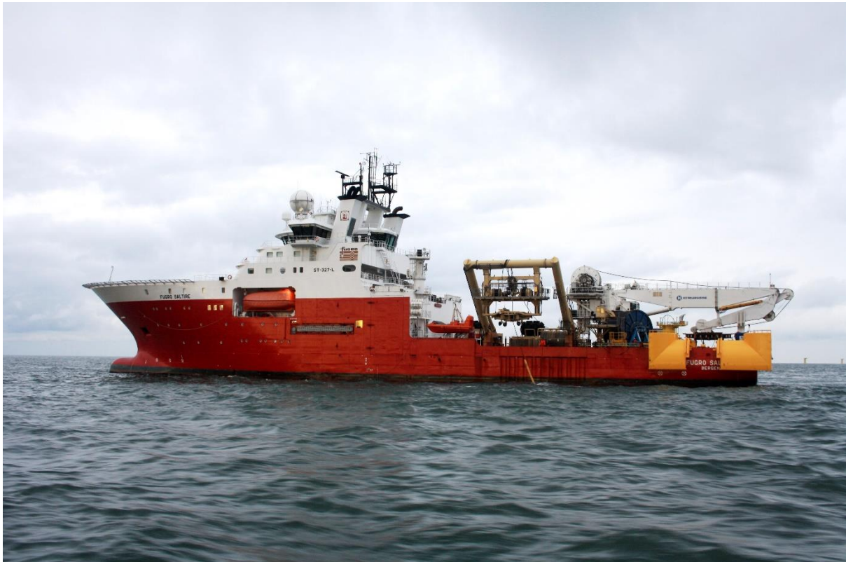
Graphic 1-4 Example array cable installation vessel (Rampion 1 offshore wind farm)
